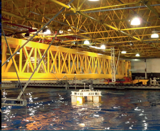
E-Semi wave basin model test in LabOceano.
